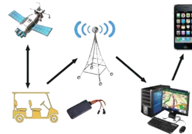
GPS Fleet tracking to enable swift and tracked movement of the shuttle vehicles
