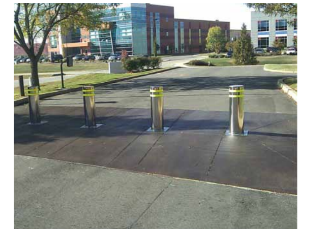
Retractable bollards which can be closed in case of crossing of emergency vehicles. Source : http://annsfasteners.com/products.html
