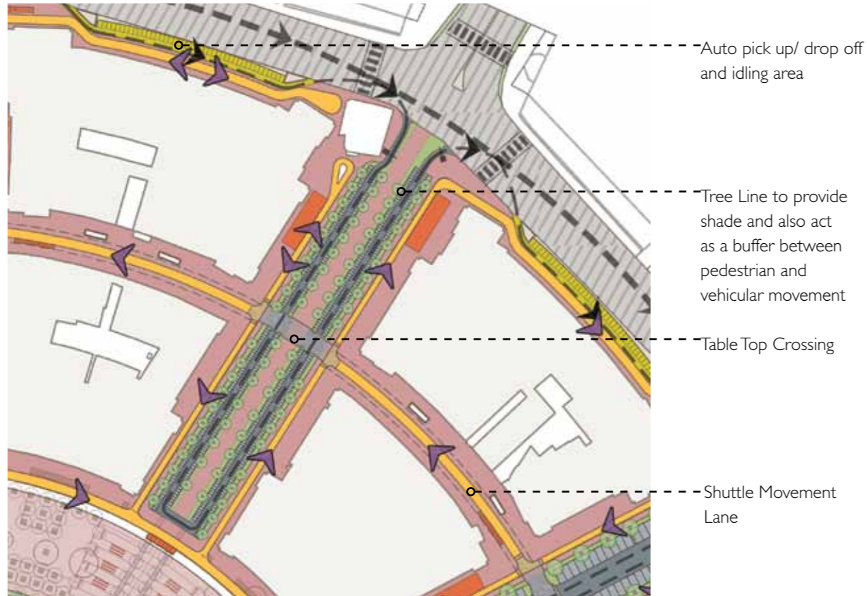
Detail of Radial 2 showing Premium Two Wheeler Parking and Movement of Shuttle
