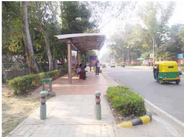
Bus stop placed on the footpath allowing continuity of the pedestrian route from behind as well as front of the shelter
